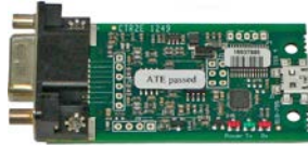
DSCUSBOEM1 The new PCB version with connectors and a 9 way D type slot and micro USB
